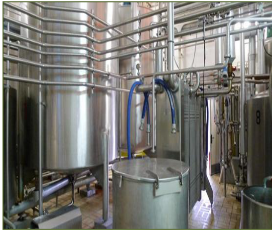
Multiple Water lines and CIP System
